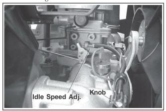
Figure 26. Carburetor and Idle Speed Adjustment.
